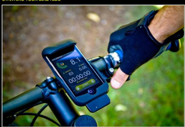
When your hardware and software setup is complete and you begin bike riding with LiveRider, the green light on the receiver should blink about once a second. This indicates that the LiveRider cycling receiver is receiving information from the sensor. As pictured here, the green chainstay icon on the main screen will say "Start" or "Resume" when the app is successfully communicating with the receiver.
